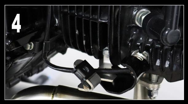
**5)** Moving to the left side front. Similar deal here to the other side. Remove the M6 bolt that secures the temperature sensor guard, fit the stay on top of the guard and refit the standard bolt.
