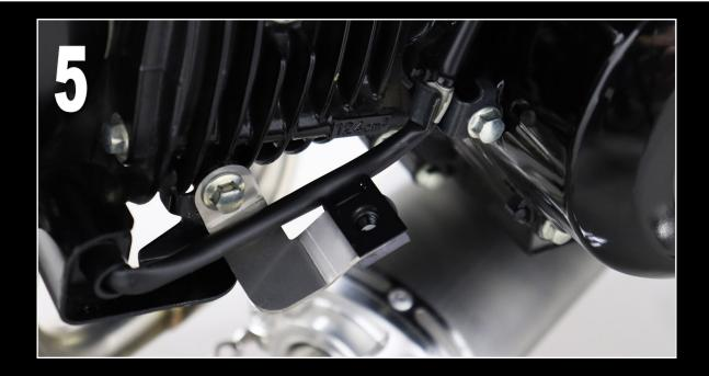
**6)** Finally, we need to swap some parts. Remove the bolt shown and replace with the rear left stay, bush and 55mm long bolt.
